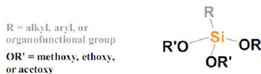
Figure 4. Silane basic structure. 58 [Color figure can be viewed in the online issue, which is available at wileyonlinelibrary.com .]
