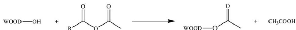
Figure 11. Reaction of wood OH-groups with acetic anhydride; Acetic acid is formed as side product.
